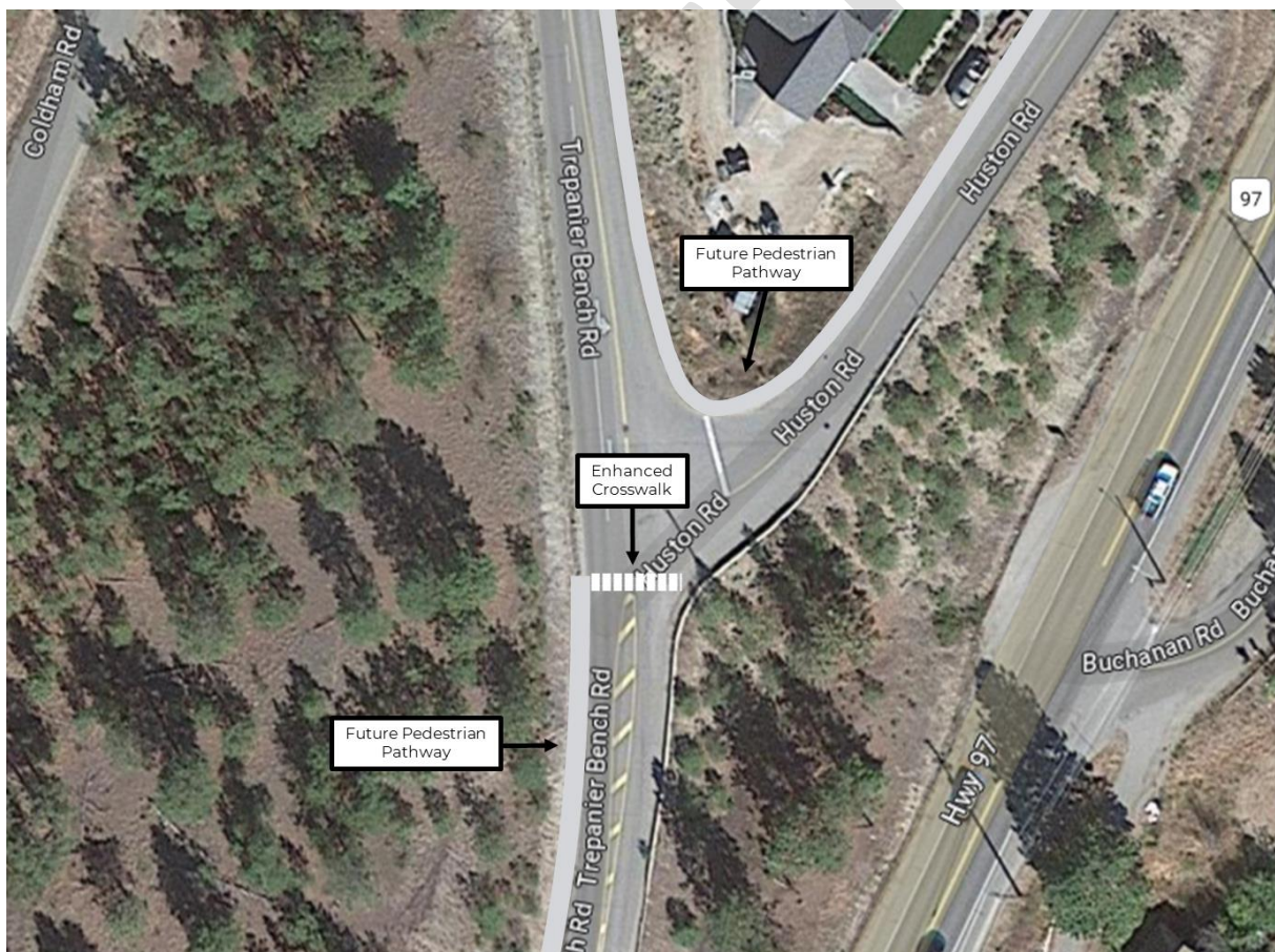
Figure 2-59: Trepanier Bench Road / Huston Road Improvement Recommendations
