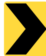
Figure 2-28: WA-9 Chevron Alignment
